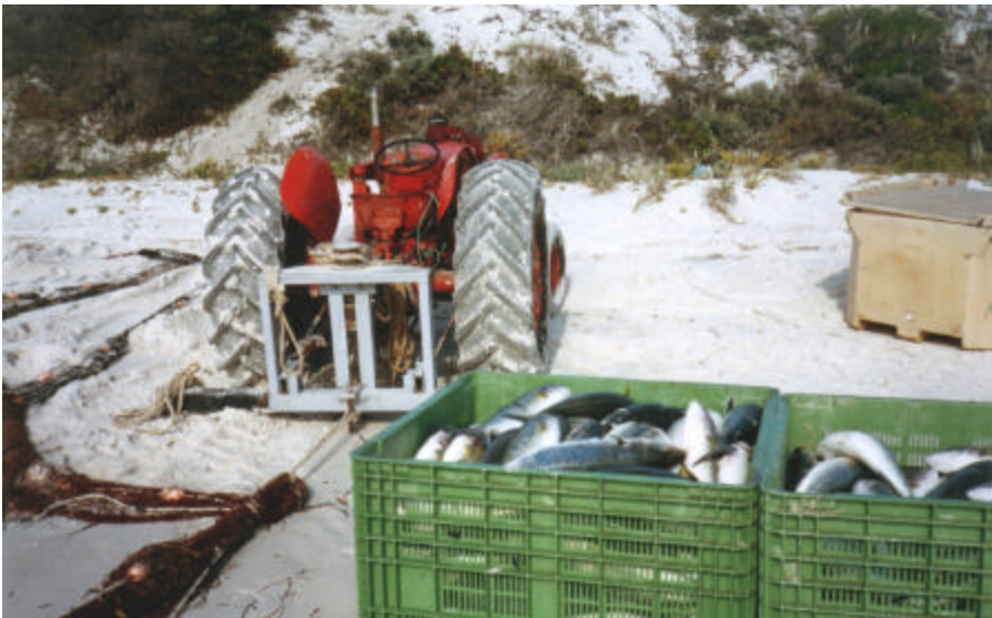
Massey Ferguson tractor, with rear mounted capstan winch. Two 0.5t bins, ice bin.
